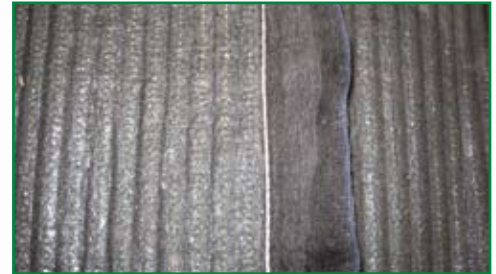
Figure 5 - FieldTurf's sewn seams with selvedge edging flap
