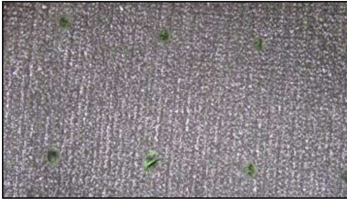
Figure 3. Example of competitor's perforated backing failure:
