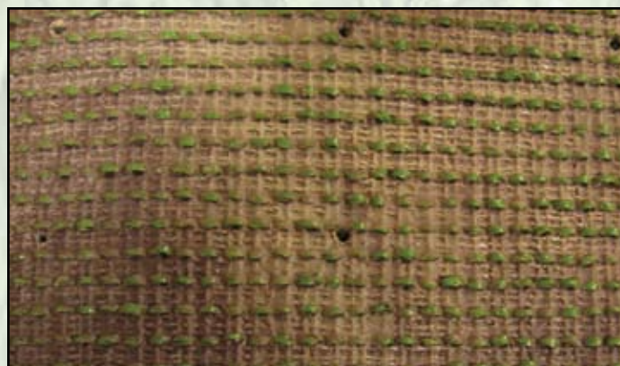
Figure 2. Competitor's perforated backing system:
