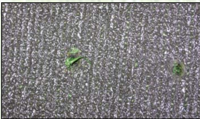
Figure 4. Close up of a competitor's clogged drainage hole
