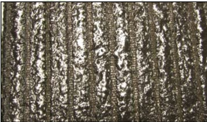
Figure 1. FieldTurf's patented finger coated backing:
